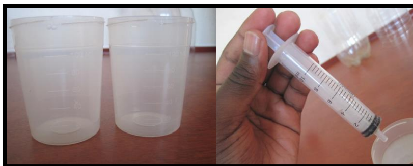
Figure 4.4 Using the volumetric flask and syringe to measure equivalent depth
