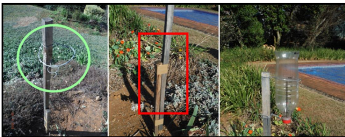
Figure 4.11 Installation of rain gauges
