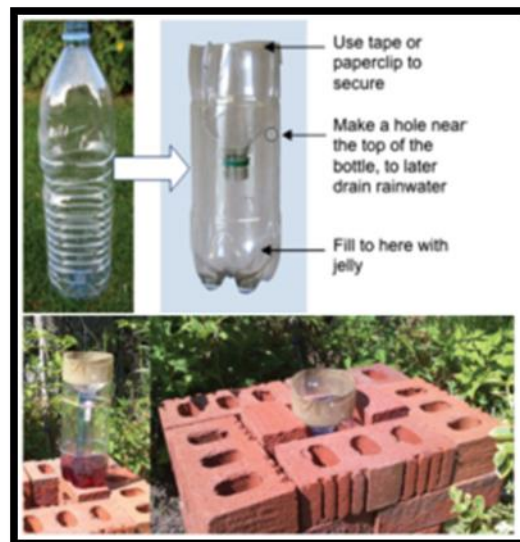
Figure 3.1 Recycled coca-cola bottle rain gauge
